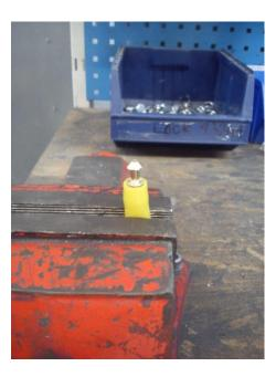
Use the guide clamp to form a joint. Fix the both ends to the tool and then close clamp (see in pictures below).
