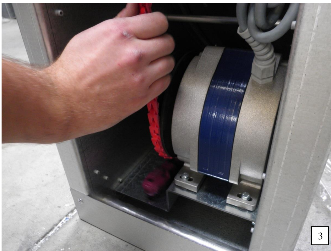
After placing the belt on a pulley turn the wheel several times to the belt properly settled.
